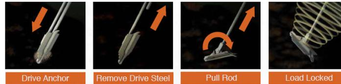
Drive Anchor    Remove Drive Steel    Pull Rod    Load Locked
